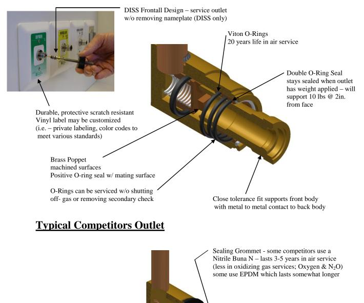
Grommet <u>deforms</u> and <u>leaks</u> when weight is applied to outlet
